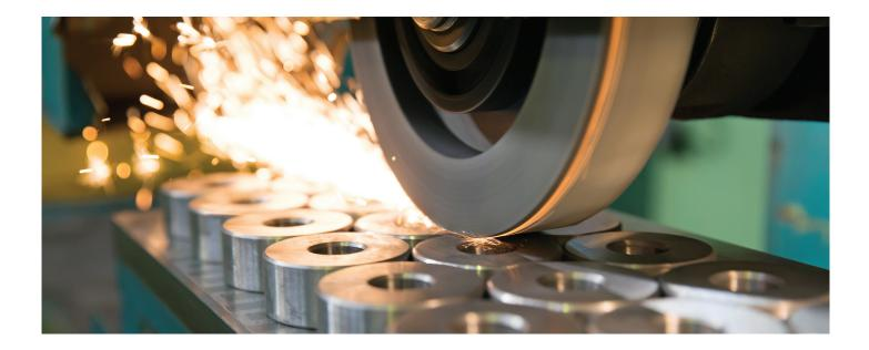
0.100" in width. However, the most widely used wheels are conventional glass-bonded abrasives, including aluminum oxides and ceramics, due to their lower cost.
