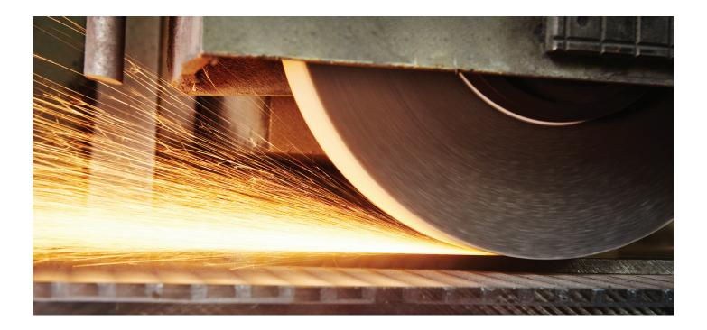
In some cases, creep feed grinding is as much as 400/0 faster than alternative processes while generating minimal burrs.
