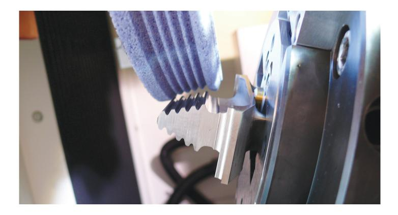
Two key challenges exist for shops considering adding creep feed grinding capability. The first is gaining knowledge and experience needed to successfully implement the process. The second challenge is justifying the cost of creep feed grinding equipment. workpiece, sends it to heat treatment, then brings it back for finish grinding, creep feed grinding can eliminate two steps in the sequence.
