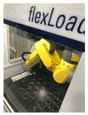
Along with production speed, safety tops the list of necessities for automation systems. For this reason, UNITED GRINDING Automation Solutions opted to create a full-system enclosure for its flexLoad with a flanged side door between the machine and the robot. Because this portal remains closed unless the machine operator issues an explicit request for entry, the system provides necessary safety precautions without using a collaborative robot.
